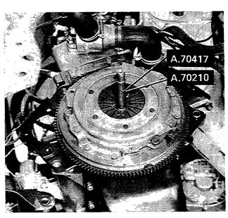
Alignment of driven plate when refitting clutch using centering pin A.70417 (1300) or A.70210 (1500 and 1600)
