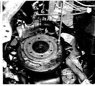
Removing clutch assembly
